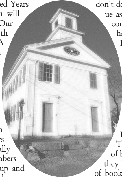
The Portersville Academy at 74 High Street is described on the National Register of Historic Places as: 1839 Portersville Academy. 2-story, Greek Revival, clapboard building. Twin front doors have simple pilasters and entablature. There is a large oval window in the flush boarding pediment. Moved from its location near the Baptist Church to this site in 1880. Used as Fifth District Schoolhouse until World War I.
